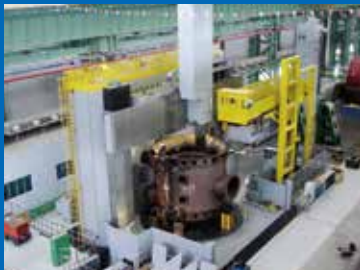
• Nine-axis five-linkage floor-type boring and milling machining center 九轴五联动落地镗铣加工中心
