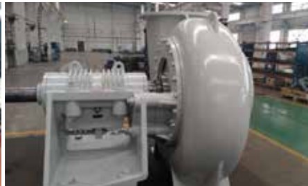
• Finished all metal desulfurization pump with the diameter of 800 800 口径全金属脱硫泵成品
