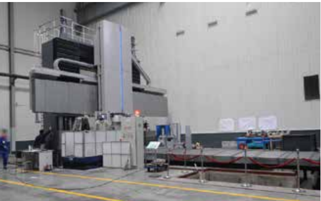
• Profimill4000/100-T six-axis five-linkage gantry boring and milling machining center ( Country: Germany ) ProfilMill 4000/100-T 六轴五联动龙门铣镗加工中心 ( 德国 )
