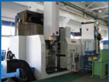
• KVL-1600ATC+CII CNC vertical turn-milling center KVL-1600ATC + C-II型数控立式车铣中心
