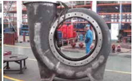
• Body of the desulfurization pump (2605N dual-phase steel) 脱硫泵泵体 (双相钢材质)
