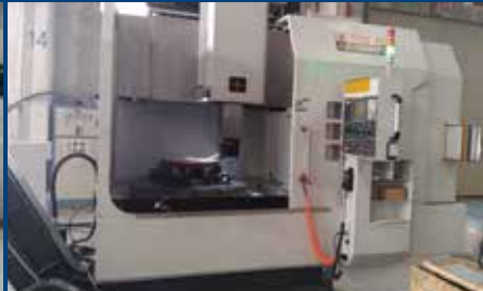
• Desulfurization Pump Guard Plate Processed through Vertical Lathe with Numerical Control 数控立车加工脱硫泵护板
