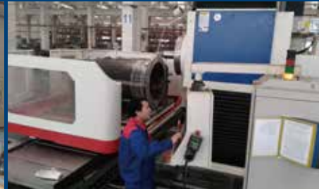
• Processed Desulfurization Pump Processed through Boring Lathe with Numerical Control 数控镗床加工脱硫泵泵体
